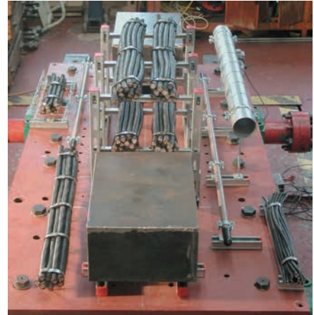
Test configuration: Two base plates were populated with MQ channel fastened with X-BT studs. The base plates were rigidly attached to the 2-tonne shock loading machine.
