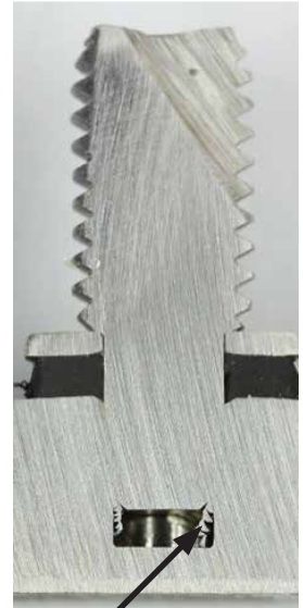
Displaced base material
