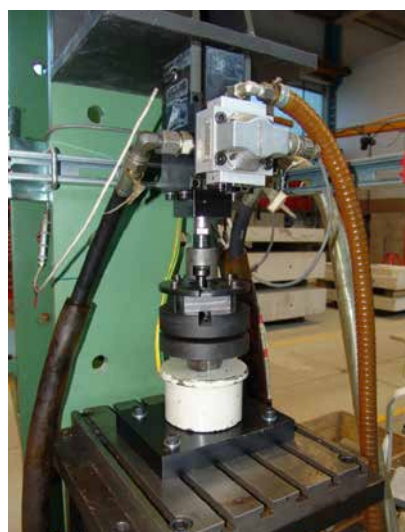
Figure 3. Servo-hydraulic test setup for tension fatigue tests
